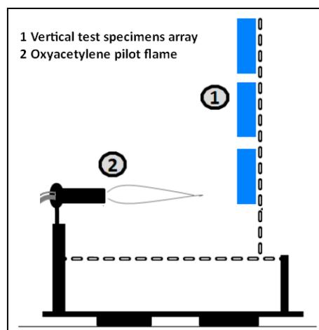
Figure 4: Experimental set-up for fire spread test.
