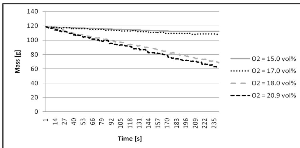
Figure 7: Test specimen mass throughout the ignition test of paper (horizontal configuration).
