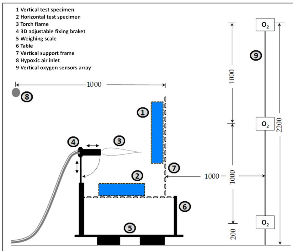
Figure 3: Experimental set-up for ignition test, horizontal and vertical configurations.
