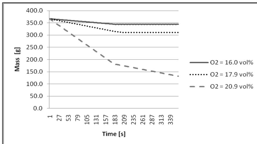
Figure 5: Test specimen mass throughout the ignition test of PP (horizontal configuration).
