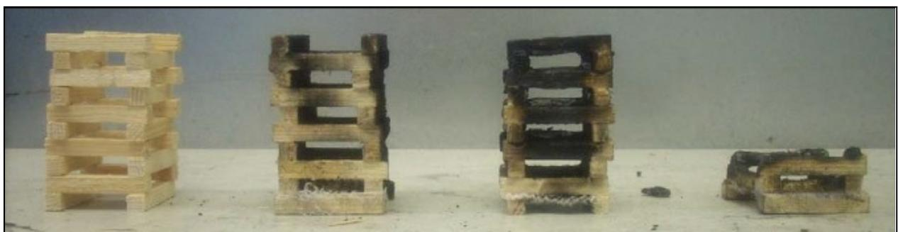
*Figure 8: From left to right: wood crib before the test, wood crib after the test at 14.9 vol%, wood crib after the test at 16.0 vol%, wood crib after the test at 17.0 vol%.*
