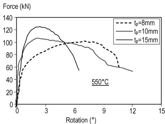
Figure 3. Effect of endplate thickness.
