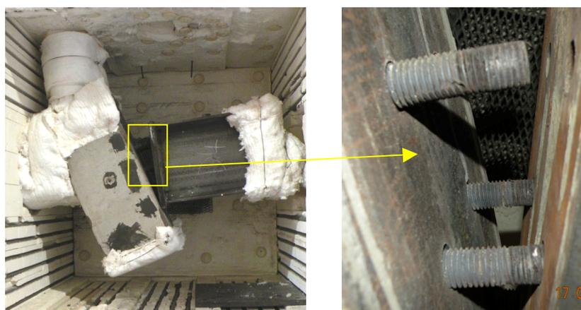
*Figure 6. Failure of flush endplate connection to partially-encased column.*
