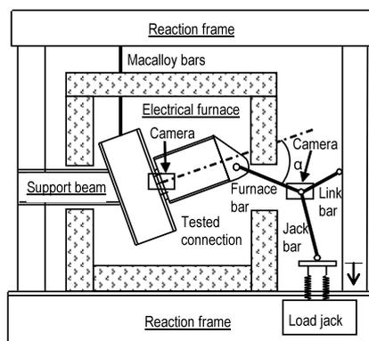
Figure 1. Test set-up.
