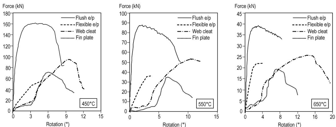
Figure 5. Behaviour of different connection types.
