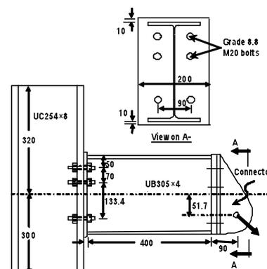
Figure 2. Typical flush endplate joint.
