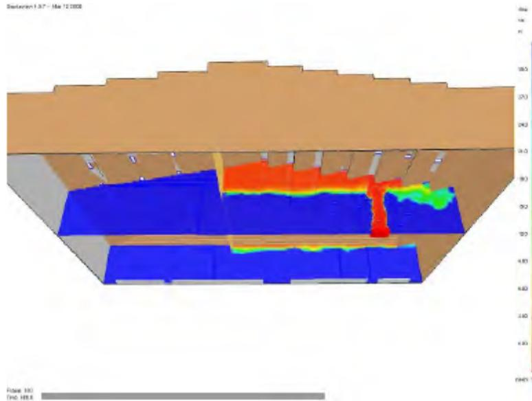
Figure 6. Results of CFD Study With Smoke Curtain Present
