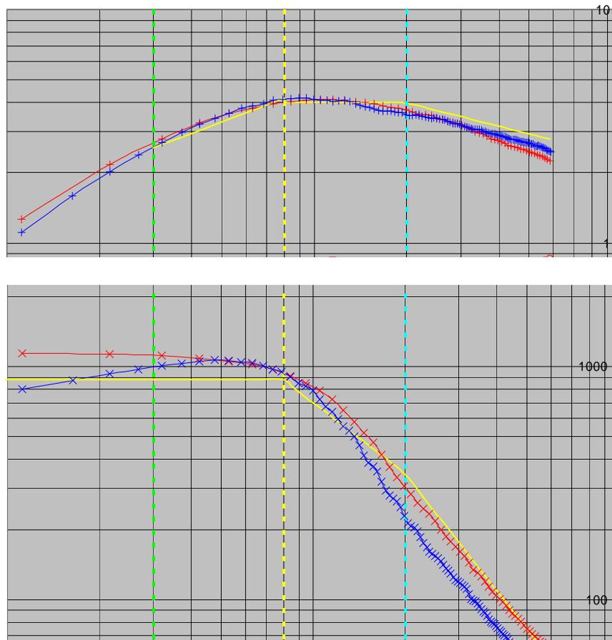
**Figure 7. Centreline mean velocity and temperature predictions using FDS [Welch (13)]**
