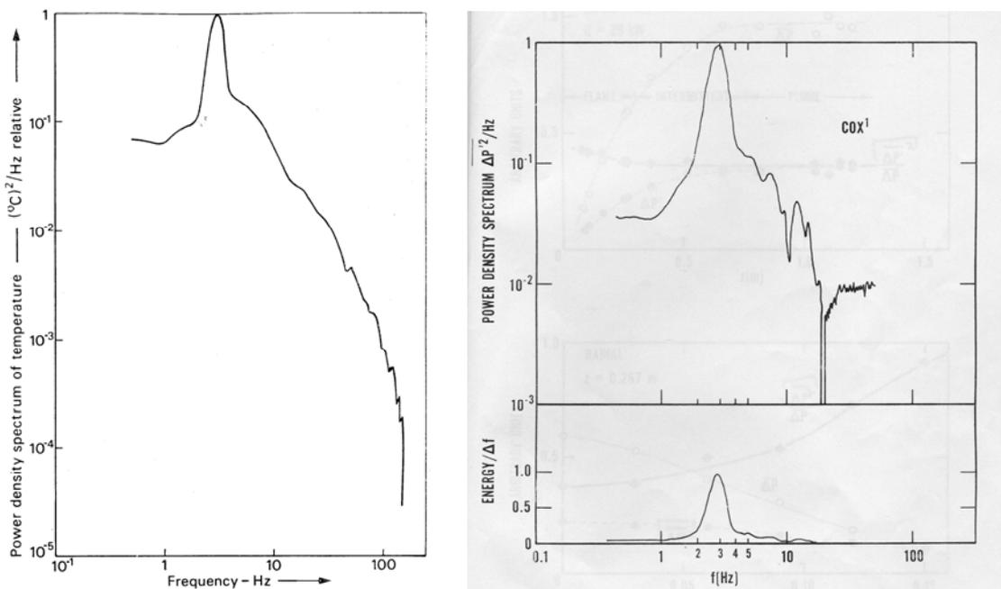
**Figure 2. Spectra of thermocouple temperature [Cox (12)] and pressure across a bi-directional probe [McCaffrey (11)] in the buoyant diffusion flame**
