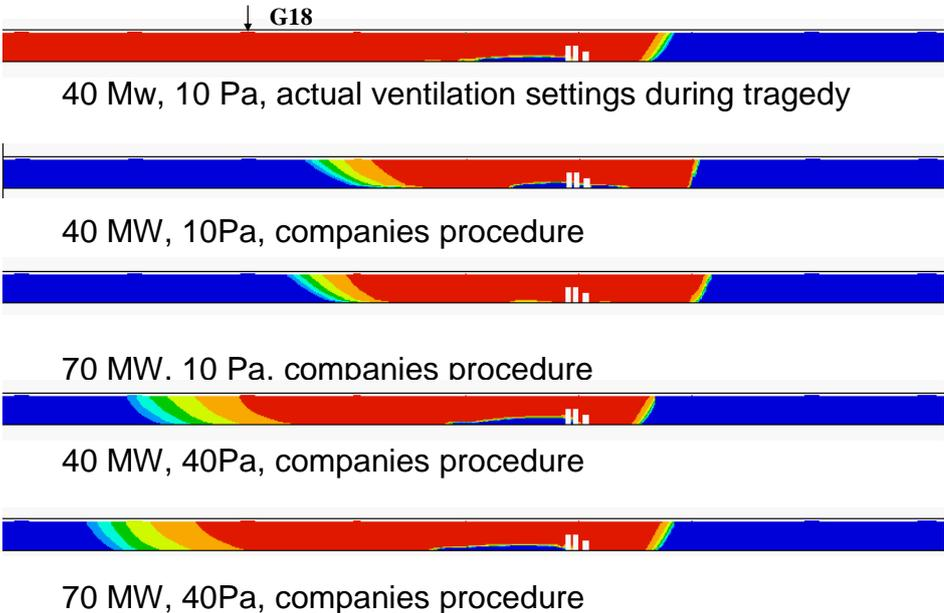
Figure 9 (b). Predictions of carbon monoxide concentration 20 minutes from ignition with different boundary conditions [21]
