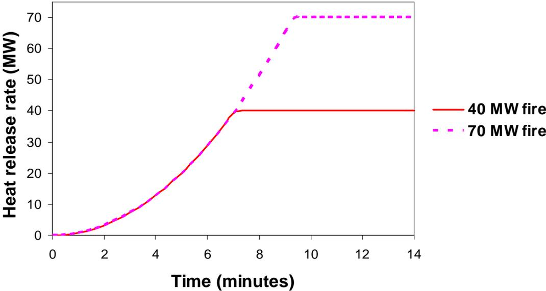
Figure 9 (a). Heat release rate assumptions used guided by witness observation and estimation
