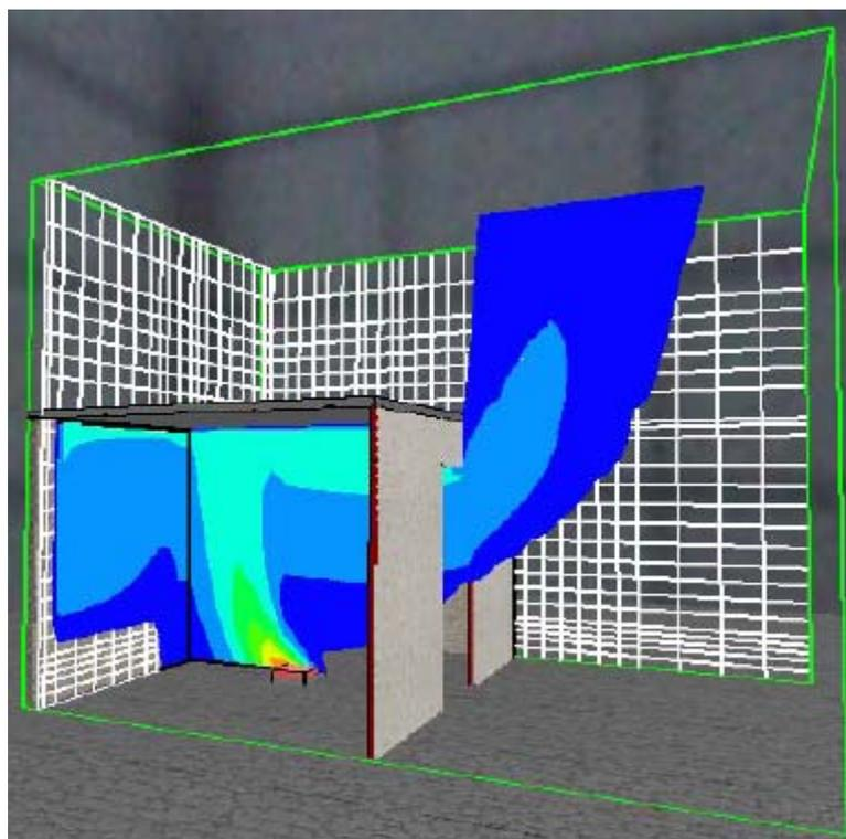
*Figure 5. Illustration of plume deflection for centrally located fire*
