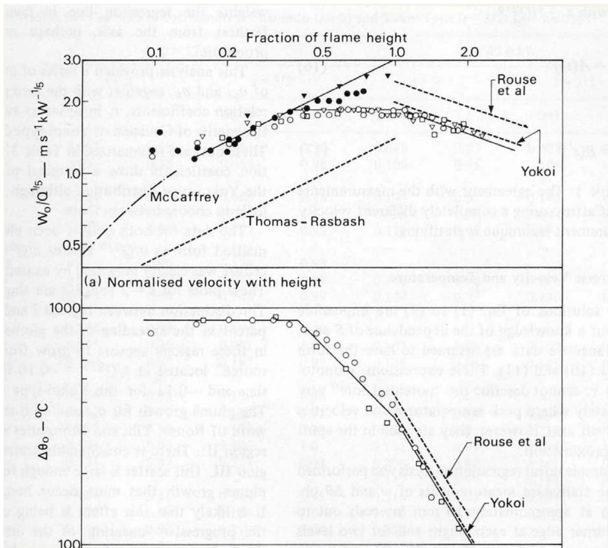
**Figure 1. Centreline velocity and gas temperature measured in buoyant diffusion flames; Langmuir probes-solid symbols; thermocouples-open symbols [Cox & Chitty (10)]**
