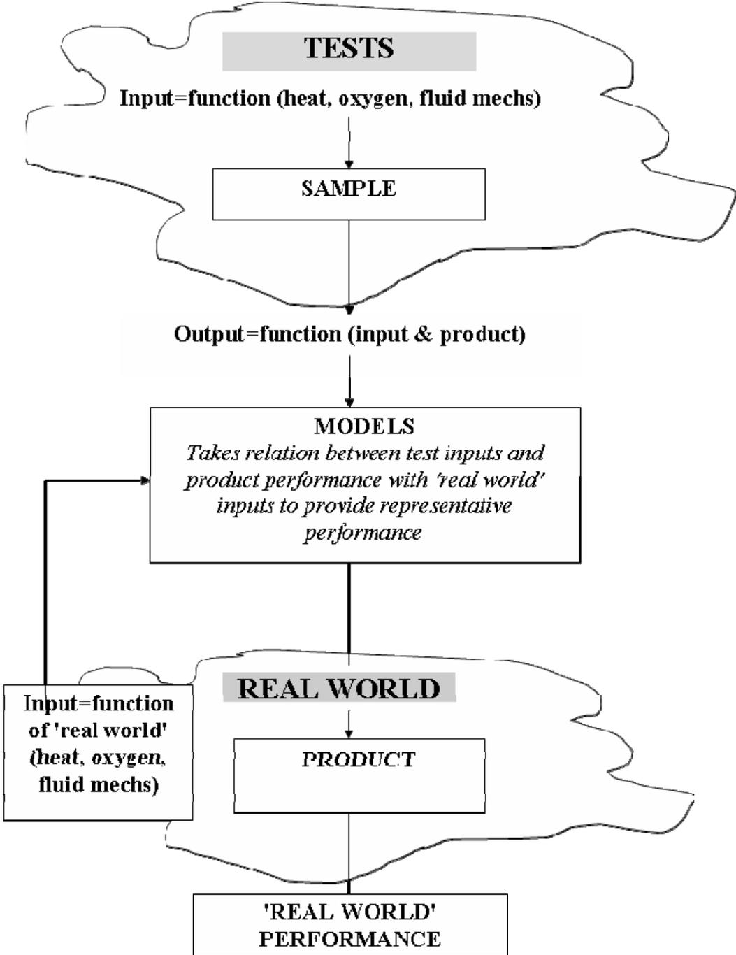
**Figure 10. Schematic Showing Proposed Role of Physical Tests and Fire Models in Fire Safety Engineering**
