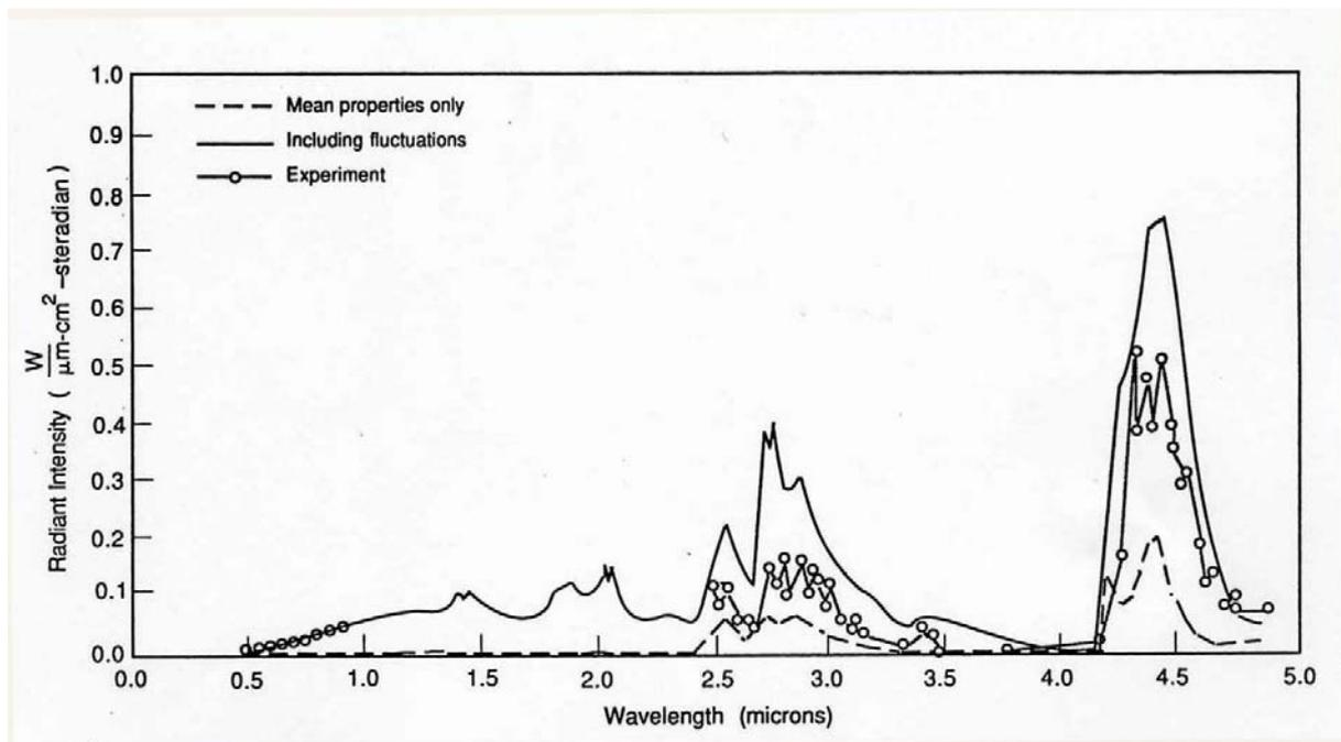
**Figure 6. Predicted spectral distribution using laminar flamelet modelling for luminous and non-luminous radiation in the buoyant diffusion flame [Syed et al (15)]**
