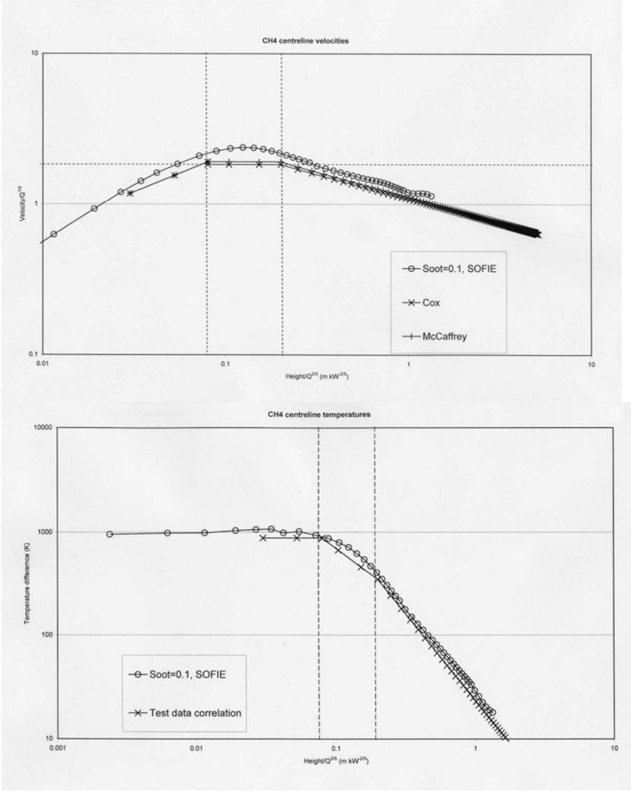
**Figure 3. Centreline gas velocity and temperature predictions by SOFIE for the buoyant diffusion flame [Welch (13)]**
