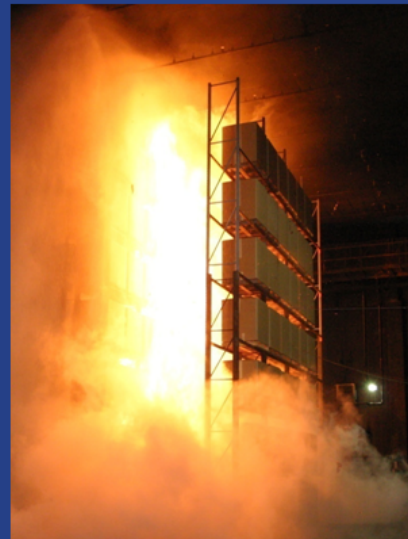
Full-Scale Sprinkler Test
