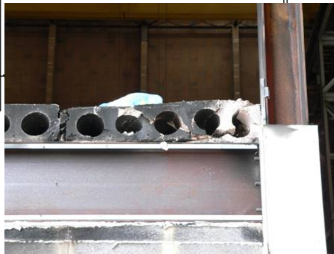
Evidence of a lateral compressive strip forming enhancing flexural and shear capacity
