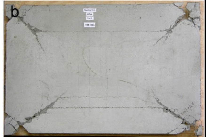
Compressive failure of concrete
