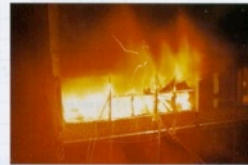
Figure 1 Fire test on a steel framed structure with a composite floor
