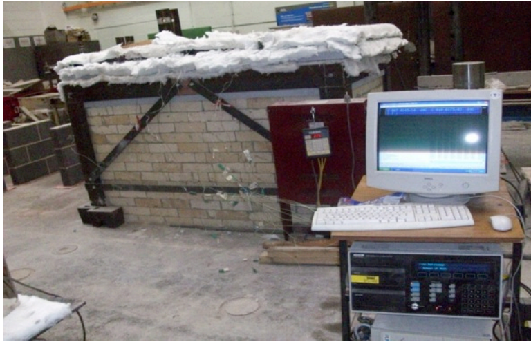
Fig.4: Electric furnace set up and columns before going in to furnace
