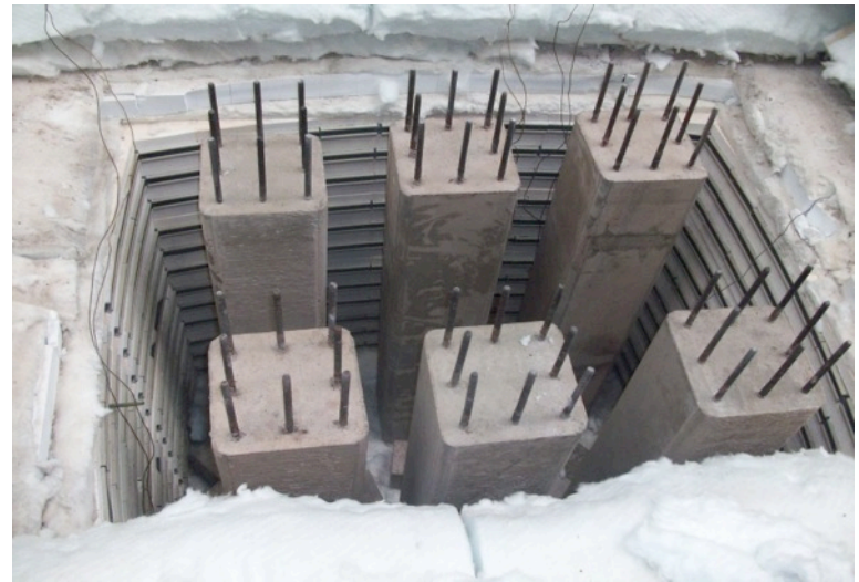
Fig.6: Columns after heating
