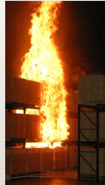
Rack storage sprinkler suppression 2012
